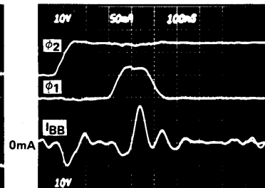
Figure 3. I_{BB} transient current during a shift cycle. I_{BB} scale: 50mA/div.
